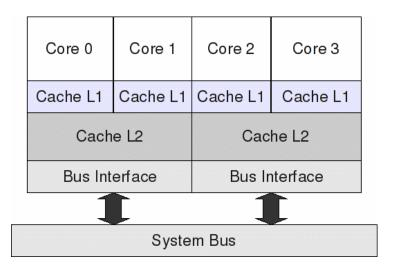
Xeon Core 2 Quad /Harpertown Two Core 2 in the same chip External main memory: shared by both L2 caches
