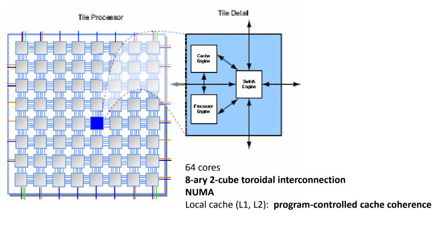
No floating-point Oriented to Video encoding, Network Packet processing
