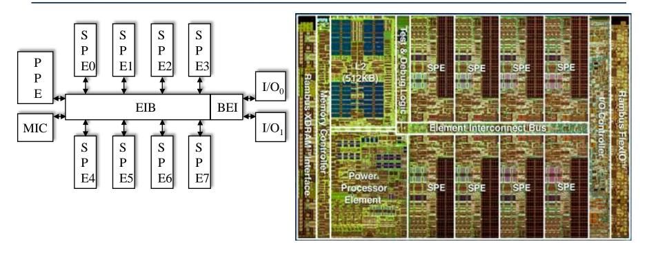
Evolution of uniprocessor (Power PC Processor Element, PPE) with 8 powerful I/O coprocessors towards a **heterogeneous NUMA** multiprocessor,
