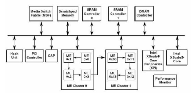
8 cores (IXP2400) or 16 cores (IPX2800), specialized for low-level packet processing,
