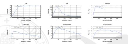
▶ In general, performance degrades when launching more threads than processors: the 4-way SMT offered by the Xeon Phi is not useful in this case.
