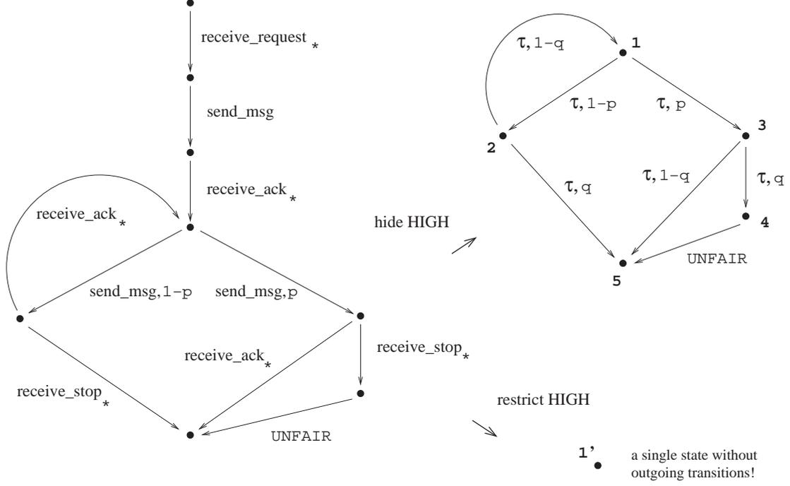
Fig. 1. Nonrepudiation protocol specification and models to be compared through equivalence checking.
