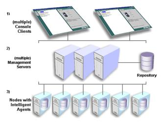
One of the most important responsibilities of the Oracle Management Server is distributing tasks to the Oracle Intelligent Agents, which run on managed nodes in the third tier. The Intelligent Agents are responsible for the localized execution of tasks and the on-going monitoring of databases and other targets on the managed nodes.
