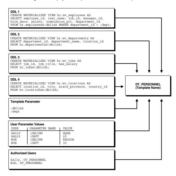
Figure 4–2 Deployment Template Elements Added to Template
