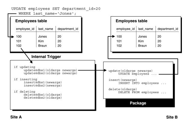
Figure 2–8 Propagating Changes Using Synchronous Row-Level Replication
