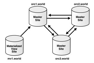
In Figure 2–3, each master site has two database links to the other master sites (N-1 or in this case 3 - 1 = 2). This configuration ensures the bi-directional communication
