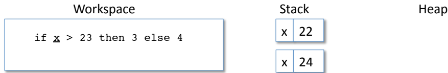
Figure 15.7: An example of how proper shadowing is implemented in the ASM. The value of the ready variable x will be found by searching the stack from most recent ( x maps to 24) to least recent ( x maps to 22).
