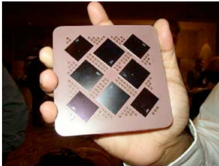
Figure 5: 8-way SMP (4 power5 chips, in the middle) with 144MB L3 cache (4 chips external)
